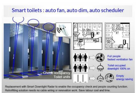
Figure 7. A Smart Toilet Use Case with radar sensors
